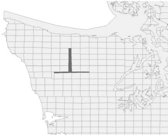
FIGURE 5.5. PLS in western Washington State highlighting unusual 1/2 townships and ranges. These peculiar townships are the results of difficulties surveying in the alpine Olympic Mountain Range. Other distortions are also plainly visible in this portion of western Washington State.
