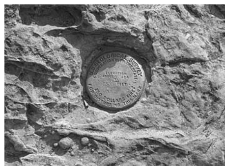
FIGURE 7.3. Geodetic markers are part of national triangulation networks and are connected to geodetic datums.
