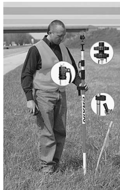
FIGURE 7.1. Professional surveyors need high-accuracy equipment such as this prism pole, which reflects the laser light used in detailed surveys.
