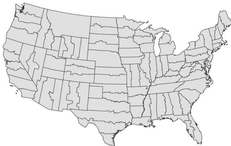
FIGURE 3.5. U.S. continental State-Plane Zones (NAD83). These zones are commonly used in the United States for state geographic information activities and are often defined by statute.
