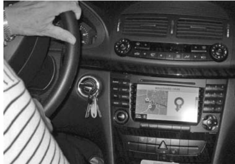
FIGURE 7.6. GPS navigation system built in as an integral part of a car's dashboard.
